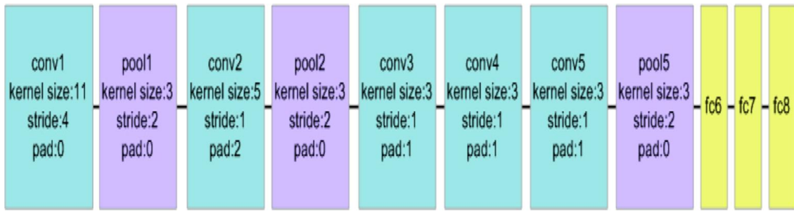
Fig. 8. Basic architecture of AlexNet
