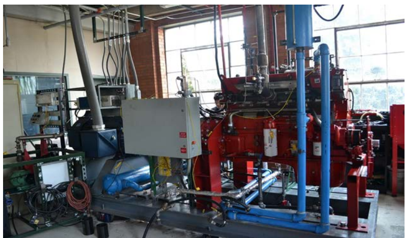
Figure 5. Cummins X15 SCE test cell.
