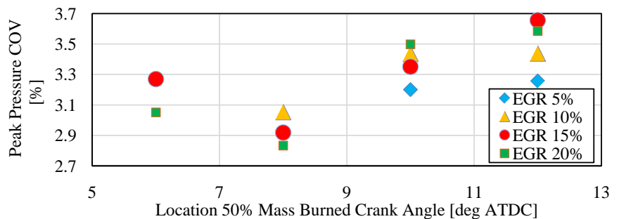
Figure 12. Location 50% mass burned crank angle vs COV and IMEP COV for different EGR ratios. Operation conditions 1200 RPM, IMEP 16 bar.
