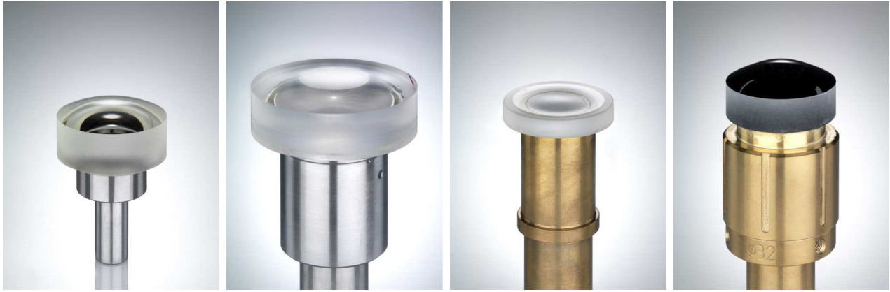
Figure 1. The specimens used in this study from left to right: asphere 1, weak asphere; asphere 2, two radii and Siemens star pattern in central part; asphere 3, containing turning point; asphere 4, strong asphere. The specimens have diameters of 39 mm, 60 mm, 60 mm, and 40 mm, respectively (see table 2).
