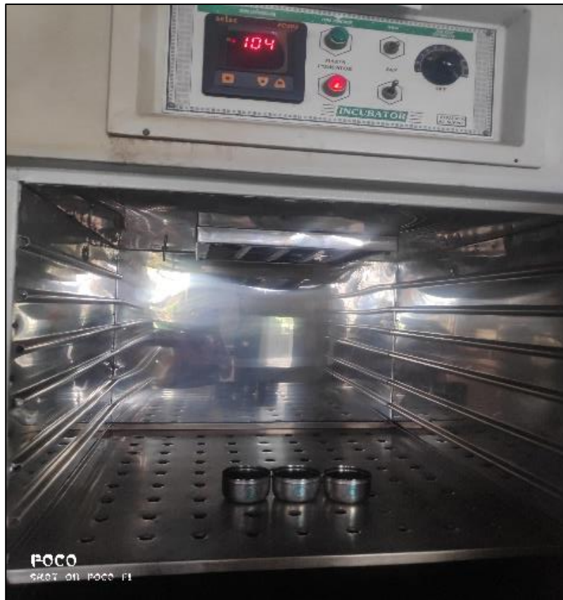
Fig. 4. Measurement of moisture content of sample using hot air oven
