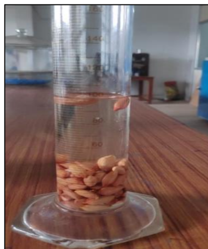
Fig. 6. Measurement of true density with toluene liquid
