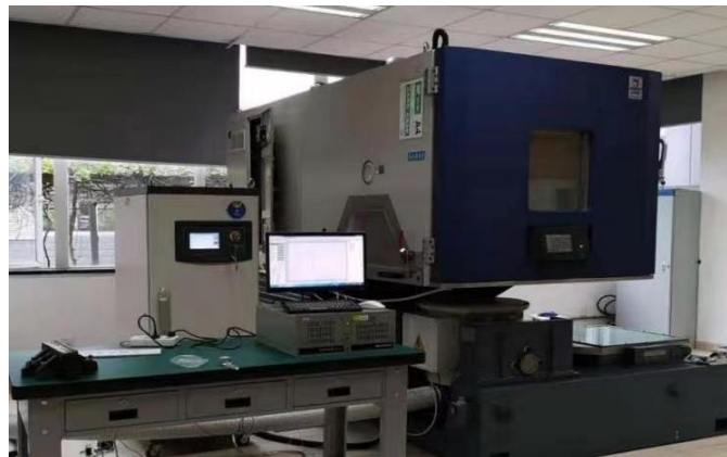
Fig. 1. Temperature rise test device of single battery
