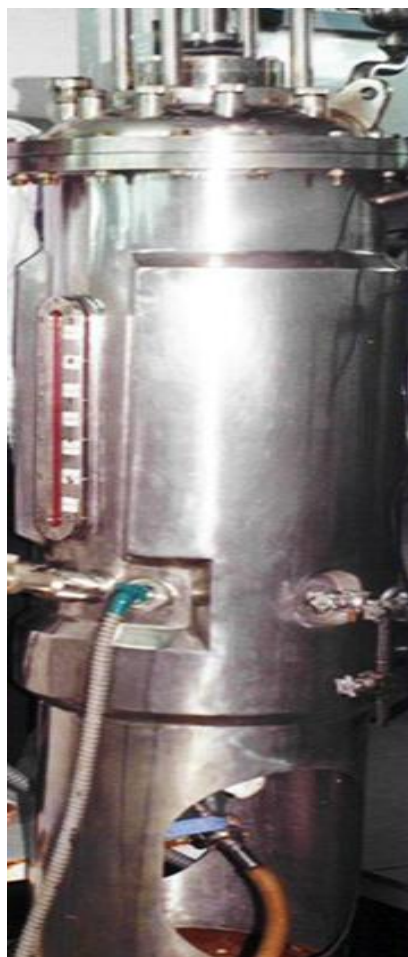
Fig. 7. Pilot-scale ajmalicine production by Catharanthus roseus suspension cultures in cost-effective culture medium in the 100 lit bioreactor
