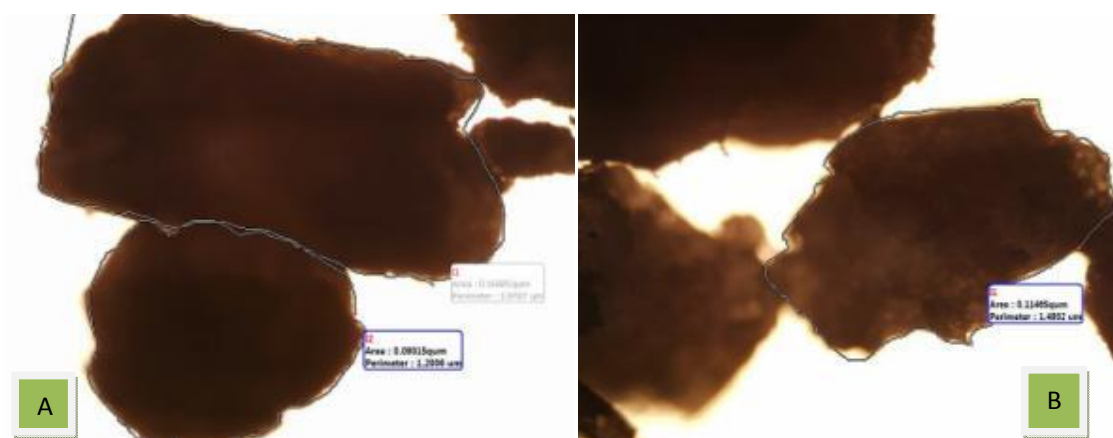
Fig. 2 a - b. Representative photomicrographs of indomethacin solid dispersions (magnification x 100)
