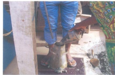
FILLING OF CONE WITH CONCRETE
