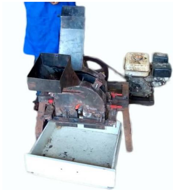
Fig. 2. The pictorial view of the portable ginger slicing machine
