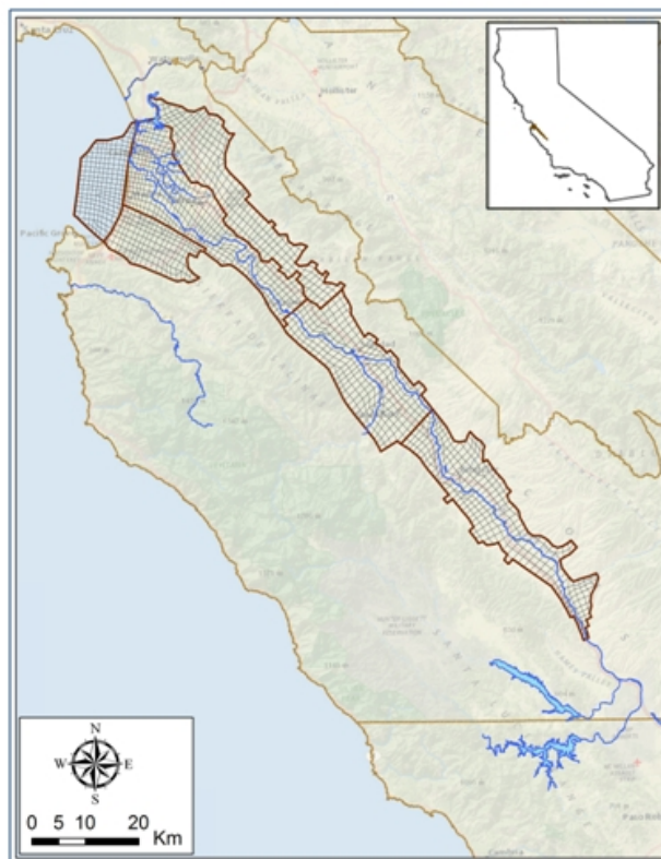
Fig. 18. Finite element grid for salinas valley model
