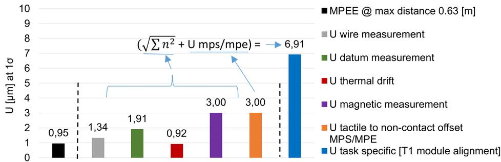
Figure 17. Final alignment uncertainty of magnetic axis alignment measurements using the three spheres datum of CLIC T1 assembly and respective quadratic contributors.
