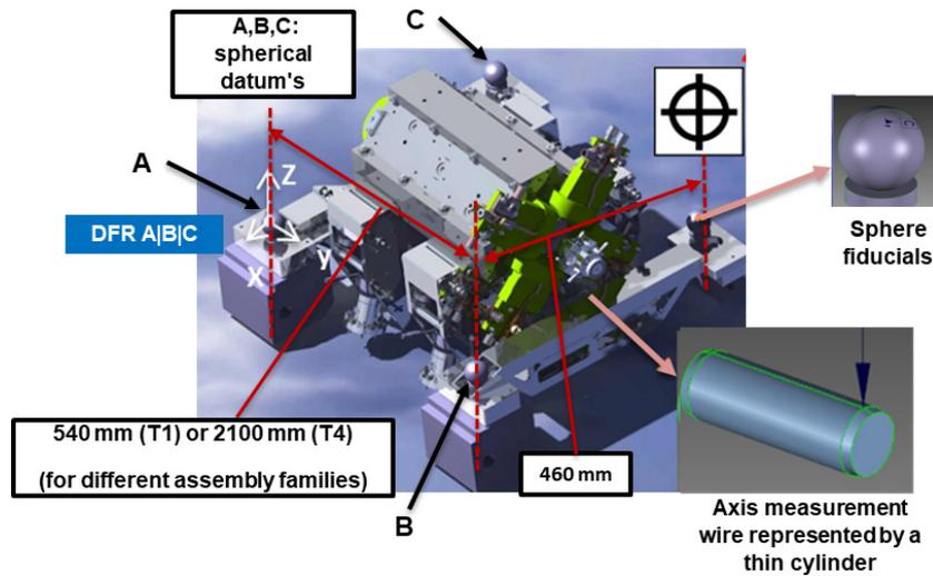
**Figure 10.** Magnet assembly and GPS language task example with four alignment fiducials.
