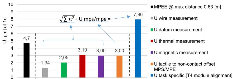
**Figure 18.** Final alignment uncertainty of magnetic axis of CLIC T4 assembly and respective quadratic contributors.
