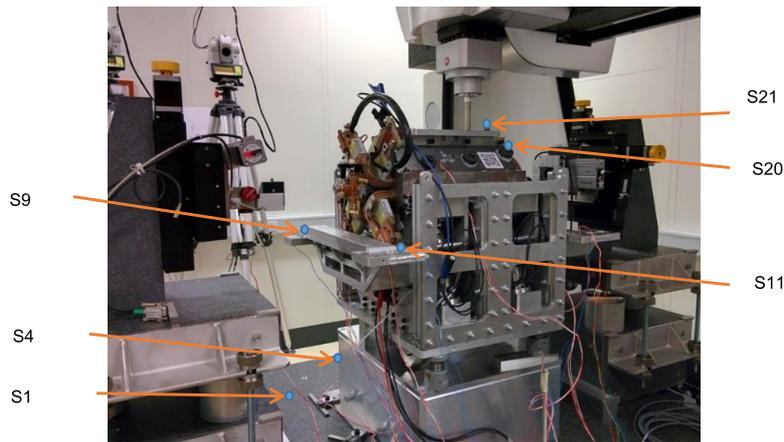
Figure 13. CLIC T1 magnet assembly integrated within CMM.
