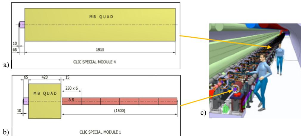
**Figure 1.** (a) CLIC special module 4 or type 4 assembly (longest magnet). (b) CLIC special module 1 or type 1 assembly (shortest magnet). (c) Sequential installation and alignment of magnets via high-precision positioning systems within the machine tunnel.
